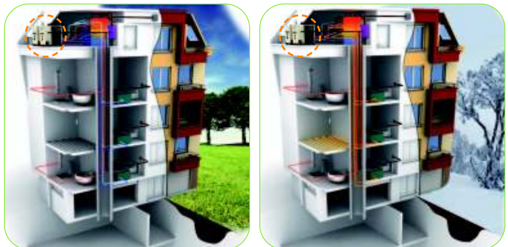
Example of GAHP-AR application in winter and summer operation for radiant panels, fan coils, indirect production of DHW.
