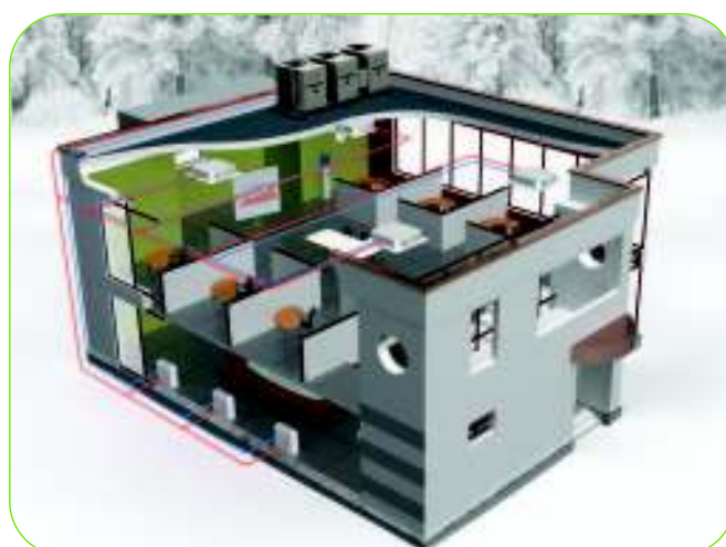
Light commercial application with fan coils and ceiling splits
